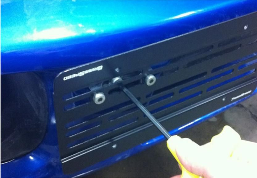
5. When the desired location of the bracket is chosen, tighten all three adjustment bolts using a 5mm hex wrench.
