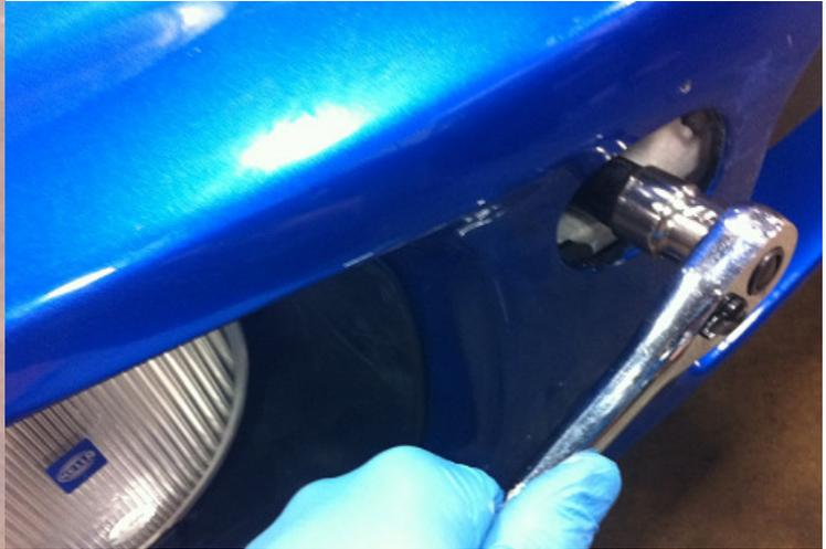
3. Depending on the model, you may need to use one or two spacers that are included in the kit to properly space the U-bracket from the bumper cover. Using the M6x25 bolt, thread it into the tow hook bolt with the U bracket and spacers (as needed) in between. The spacers (as needed) will be placed between the tow hook bolt and the U bracket. Loosely tighten with a 5mm hex wrench.
