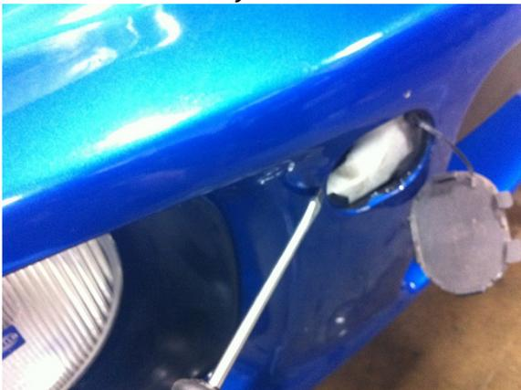
2. Apply grease or anti seize to tow hook bolt. Using a 17mm socket, tighten the bolt to approximately 45 ft. lbs.
