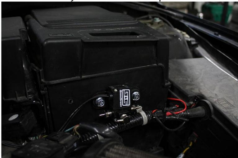
7. Disconnect brake booster vacuum line for easy access to solenoid.
