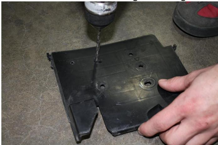
6. Using provided Grimmspeed bolts and nuts, mount the solenoid on the battery cover. Reinstall battery front cover and top cover.
